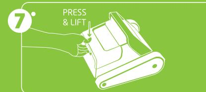
To access to the cleaner's filtering tray, do not force the access door, you must press and lift the cover.
