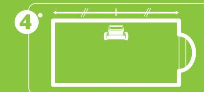
Position yourself in the middle of the long length of your pool. Put the cleaner in the water face down against the wall, and help it to evacuate the air. Make sure the cleaner stays flat on the bottom of the pool.
