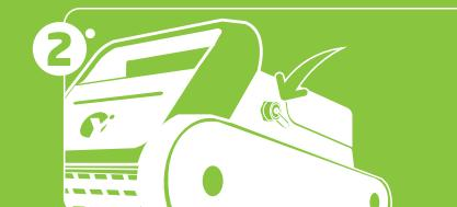
Please check that the waterproof charge cap is tightly screwed before putting the pool cleaner in the water.
