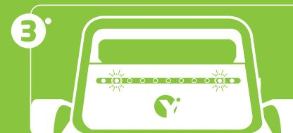
Place the robot on flat ground and wait (50 seconds) that the yellow lights are flashing before putting it in the water.
